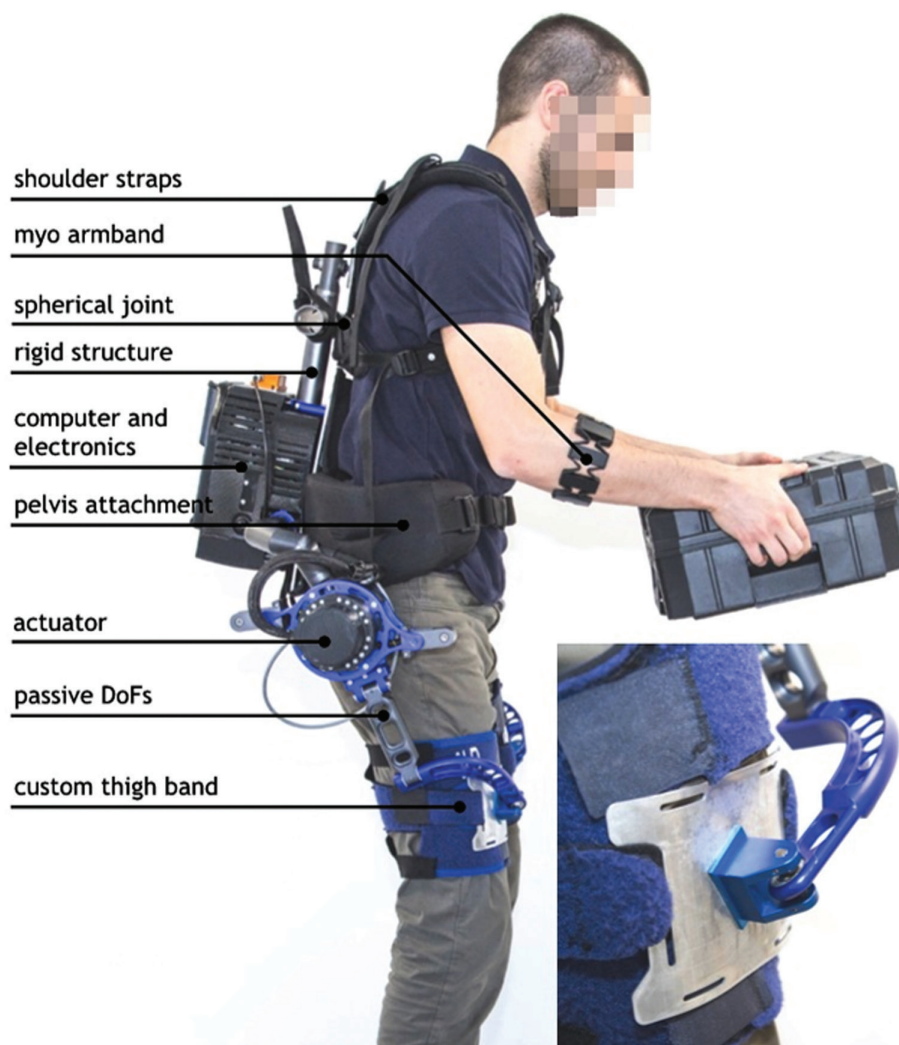
Figure 9. Wearable robot developed by the SPEXO team [146] . Copyright 2018, The Authors.
